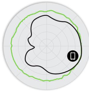
Figure 4. A510 2.4GHz Elevation Antenna Patterns
