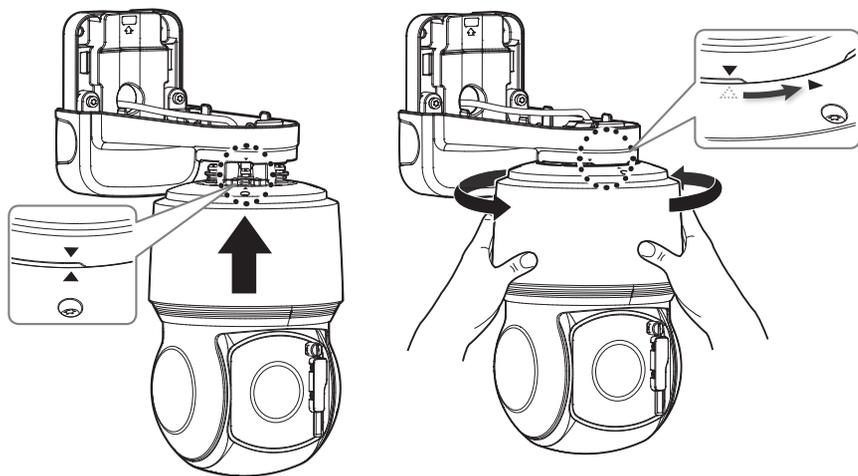
7. Join the top cover of the wall & pole mount.
