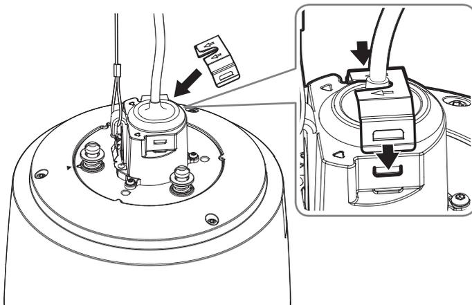
6. After aligning the installation direction guides of the hanging mount, push the main cover upward and turn it counterclockwise until it is secured.
