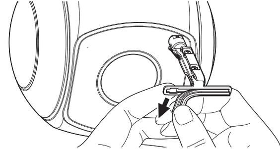
4. Insert the rubber replacement in the joint groove by sliding it in the direction of the arrow.
