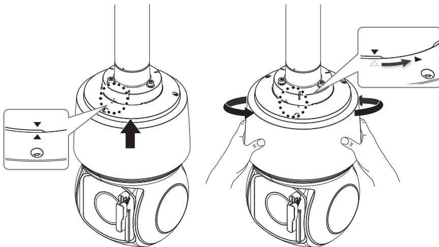
7. Tightly fasten the 3 mounting screws on the top side of the Hanging Mount.
