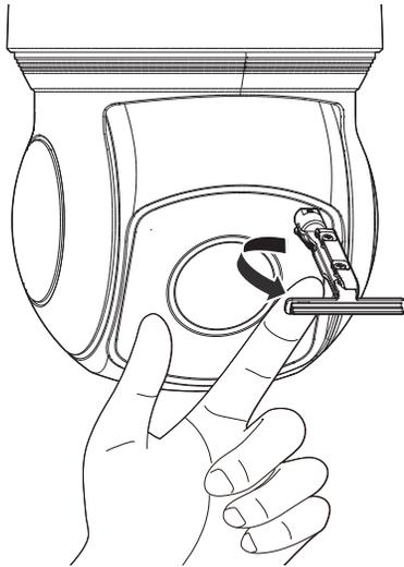
3. Remove the rubber part by pulling it back.
