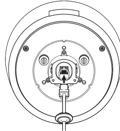
4. Plug the cable bushing of the network cable in the hole.
