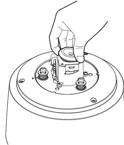
2. Pull off the extruded part of the removed cable bushing.
