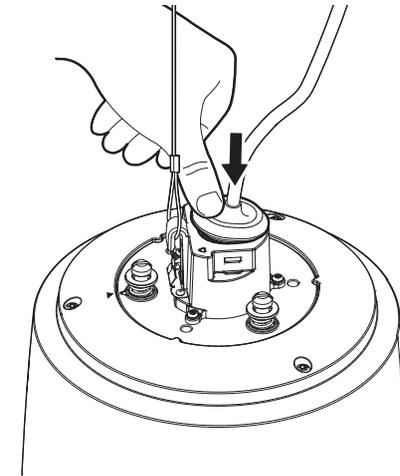
**!** The length and width of the cable bushing are different. Check the shape and plug it in the right direction.
