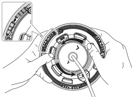
2. Remove the middle cover by lifting it.
