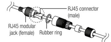
4. Assemble by rotating the RJ45 modular jack (female) and the RJ45 protection cover clockwise (Follow the arrow).
