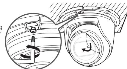
7. Push the colored camera part upward in the direction of the arrow, and tighten the screws in the direction perpendicular to the ceiling.
