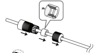
2. Connect the LAN connector (male) to the cable.
