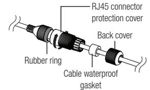
5. Assemble by rotating RJ45 protection cover and back cover clockwise (Follow the arrow).
