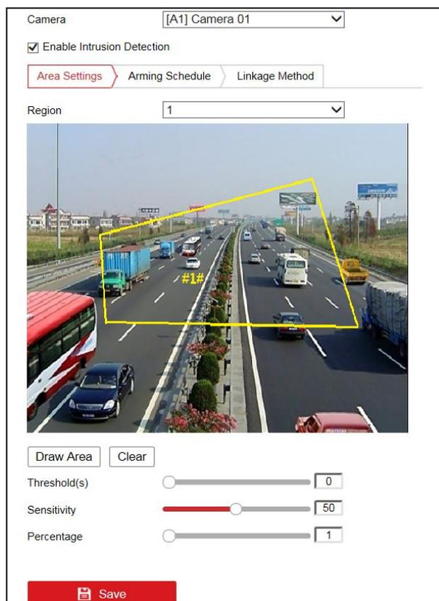
Figure 7. 14 Intrusion Detection
