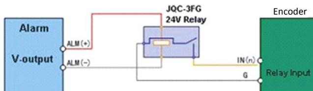
Figure 1. 5 Alarm Input Connections for Normal Alarm
