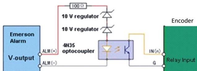
Note: The relay input port of the Encoder should be set to NC mode.
