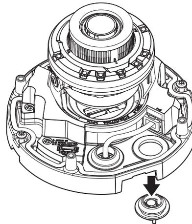
7. Insert the cable bushing of the audio/alarm cables into the camera body.
