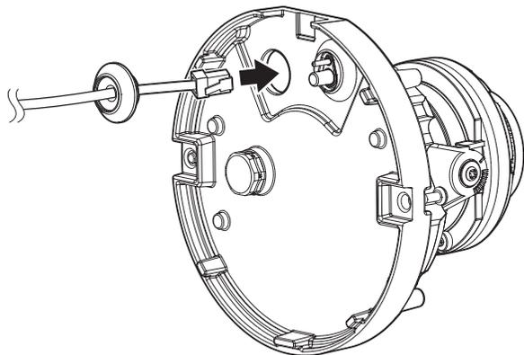
5. Connect the network cable connector to the PoE port of the camera body.
