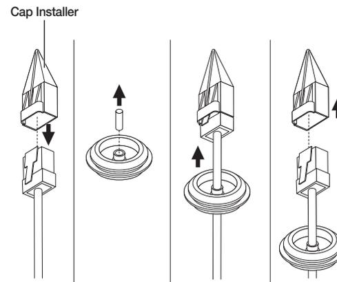
4. Insert the cable bushing of the network cable into the camera body.
