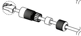
3. Connect the RJ45 modular jack (female) to the RJ45 connector (male).
