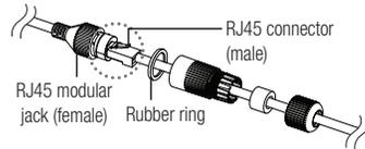
4. Assemble by rotating the RJ45 modular jack (female) and the RJ45 protection cover clockwise (Follow the arrow).
