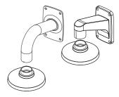
2. CEILING MOUNT ADAPTOR(SBP-300CM)/HANGING MOUNT(SBP-276HM) This adaptor is used when installing the dome camera on a concrete ceiling.
