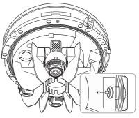
4. Use the Cap Installer to allow the RJ45 cable to pass through.
