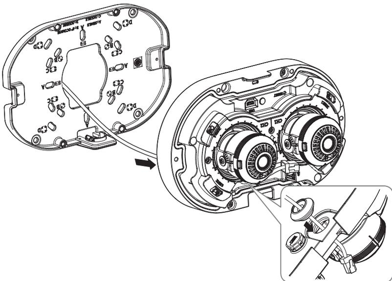
2-4. Connect the network cable jack to the PoE+ port of the camera body.
