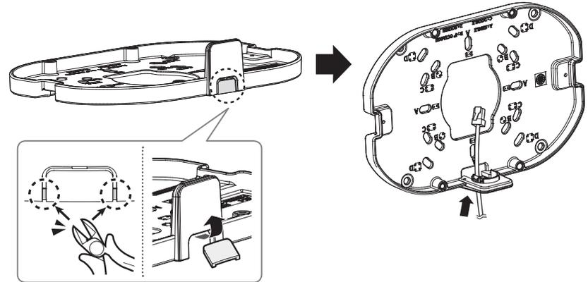
1-3. Pull out network cable through the hole in the mount plate.
