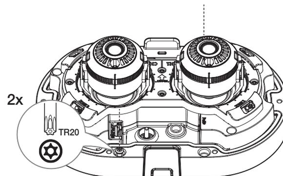
3. Separate the camera body from the mounting plate.
