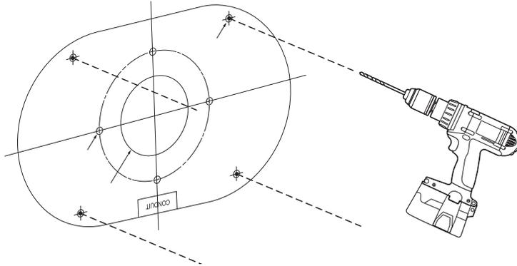
1-2. Fix the mount plate using appropriate screws.
