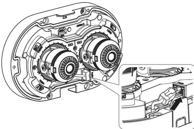
3. Using the fastening screws on the camera body, fix the camera body to the mount plate.
