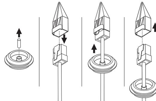
2-3. Mount the cable bushing to the camera body.
