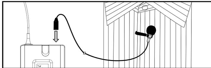
**Important Note:** Due to the distance between the talker's mouth and the microphone, lavalier microphones are not designed for use in spaces where the talker is being reinforced in the same room - such as training rooms. Using them in these applications will often result in feedback due to the higher gain necessary for proper pickup. For these applications, the single ear hook and double ear hook microphones are recommended.
