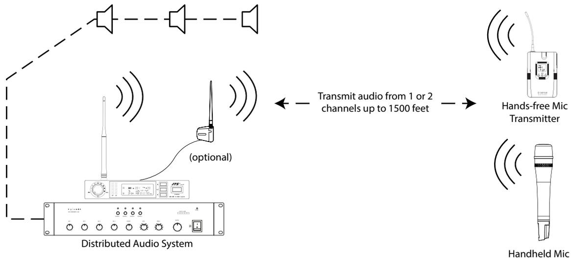
The wireless receiver can be placed on a surface or mounted in a rack. The antennas can be mounted in the front, rear, or extended with an antenna booster (sold separately) for wireless sound pick up from a handheld microphone transmitter or a hands-free body pack (see below for full list of accessories). The SE-300-WR-1CHD receives transmissions up to 1500 feet, then outputs into a distributed audio system.
