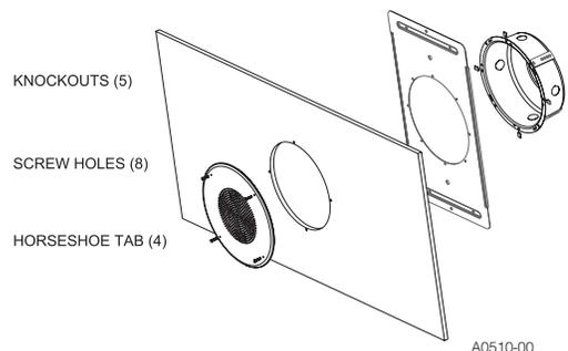
Ceiling-Mount Speaker with Back Can and SB-SPC8 tile bridge
