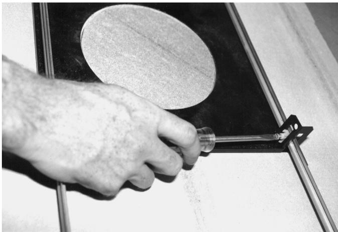
**Figure 9.3: Tighten Bracket Securing Screw**
