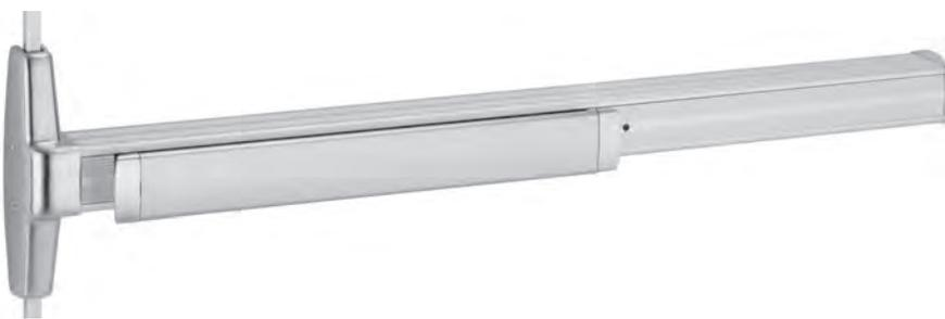
**3327A and 3527A** for all types of single and double doors, UL listed for panic exit hardware. Devices are ANSI A156.3 – 2008 Grade 1. The 3527A has a smooth mechanism case and the 3327A has grooved case. The surface vertical rod device is non-handed except when the SS (signal switch) option is used. See opposite page for available outside trim and device functions.
