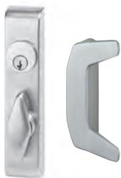
Standard operation, key locks and unlocks thumbturn. Optional operation, key unlocks thumbturn, re-locks when key is removed. This operation is created by changing the cylinder plate included with control. Use 1 1/2" mortise cylinder with a straight cam. Schlage cam reference B502-191. Not available for 3349/3549 devices.
