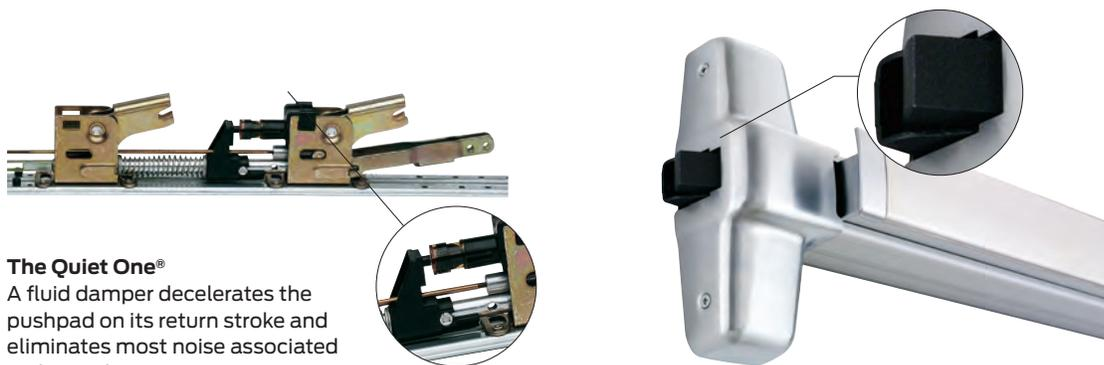
A fluid damper decelerates the pushpad on its return stroke and eliminates most noise associated with exit device operations. Furnished on all 98/99™ Series exit devices.
