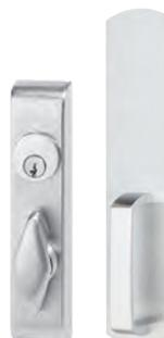
Standard operation, key locks and unlocks thumbturn. Optional operation, key unlocks thumbturn, re-locks when key is removed. This operation is created by changing the cylinder plate included with control. Use 1 1/4" mortise cylinder with a straight cam. Schlage cam reference L583-475. Use with a pull trim (990DT pictured).
