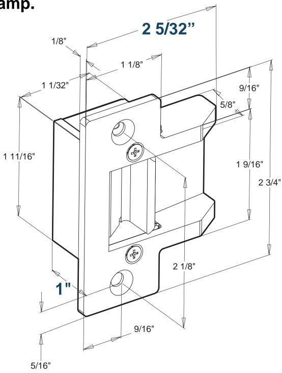
NOTE: USE 2 INCH LONG (OR LONGER) WOOD SCREWS FOR MOUNTING IN WOOD FRAMES
