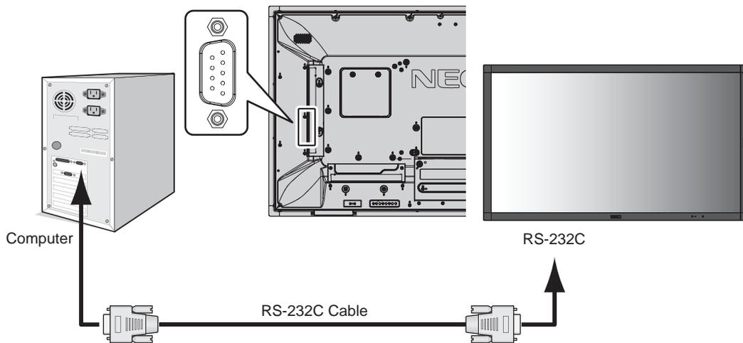
**NOTE:** If your computer is equipped only with a 25-pin serial port connector, a 25-pin serial port adapter is required. Contact your supplier for details.
