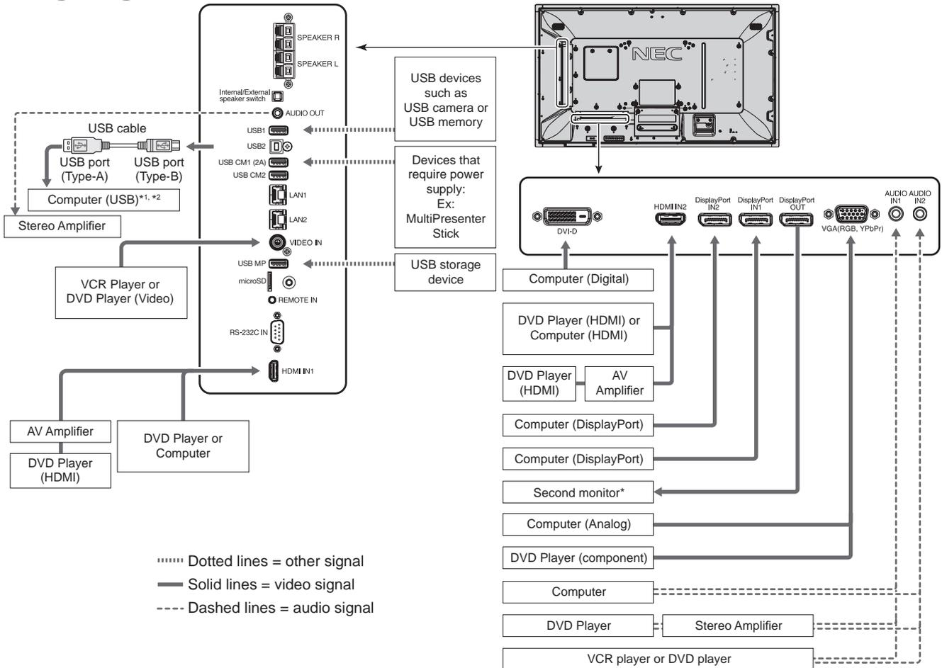
\*: Multiple monitors that are daisy-chained have a limit to the connectable monitors.
