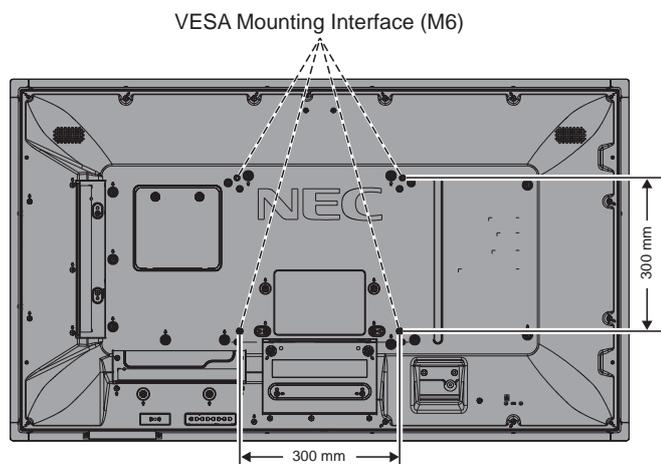
Mounting accessories can be attached with the monitor in the face down position. To avoid scratching the LCD panel, always place a soft cloth, such as a blanket that is larger than the monitor's screen area, on the table before laying the monitor face down. Make sure there is nothing on the table that can damage the monitor.
