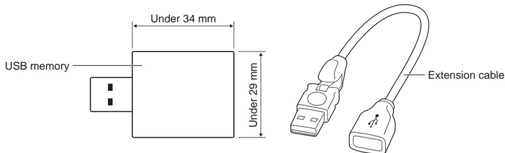
**NOTE:** Check the format if this device cannot recognize the connected USB memory. It is not guaranteed to work with all USB memories sold commercially. Please connect the USB memory to USB MP (See page 18).
