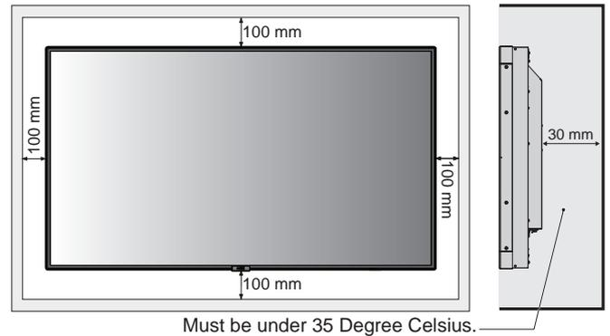
Allow adequate ventilation or provide air conditioning around the monitor, so that heat can properly dissipate away from the unit and the mounting equipment; especially when you use monitors in a multiple screen configuration.
