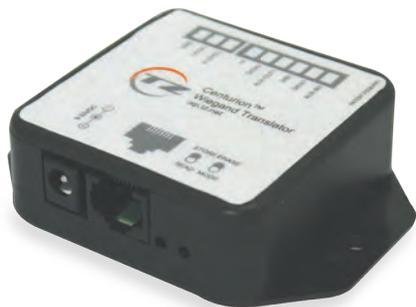
The TZ Centurion Wiegand Translator device connects to a TZ Centurion network and provides access control by interpreting a Wiegand data stream from third party credential readers such as RFID and biometric scanners. The device also provides a constant 12V DC output to power the third party credential reader.
