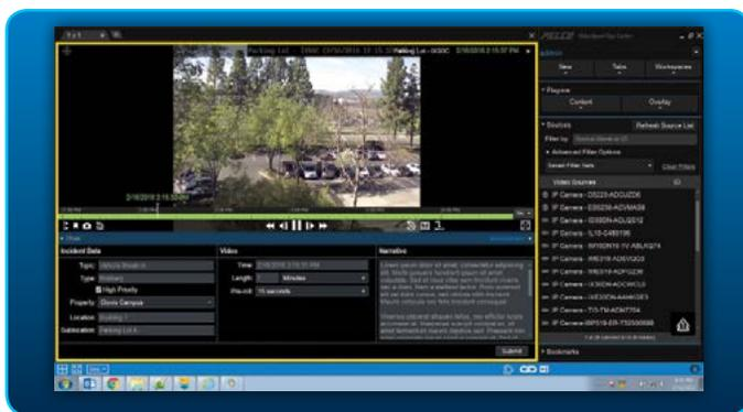
When monitoring an incident, the user interface can play a role in how quickly information is retrieved. Users can leverage the Tagging feature in the VideoXpert Ops Center to tag cameras to quickly identify cameras linked to the iTrak system. Users can select from alternative UI views to only show an incident when needed.
