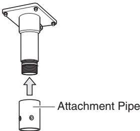
(2) Fix the attachment pipe to the bracket.
