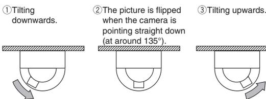
Digital flip is performed only when the system controller joystick is held downwards.
