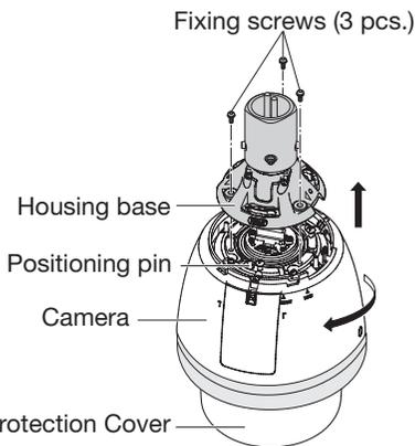
Poorly tightened screws may result in water leaking into the camera or possible fire.
