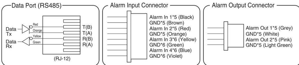
\*5: The type of twisted pair cable is AWG#28.
