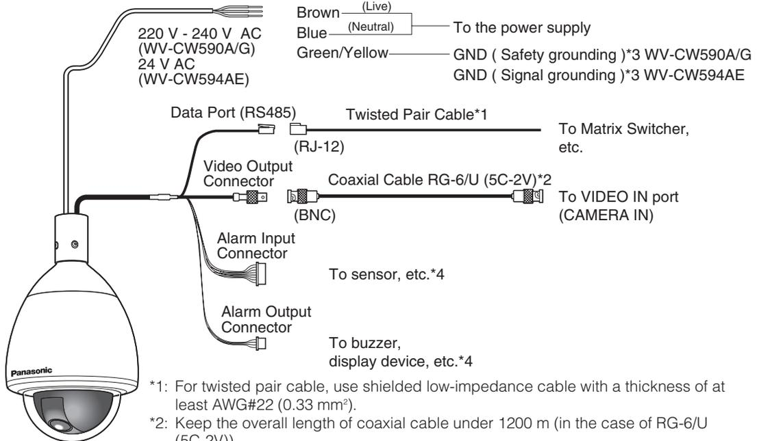
\*1: For twisted pair cable, use shielded low-impedance cable with a thickness of at least AWG#22 (0.33 mm<sup>2</sup>).
