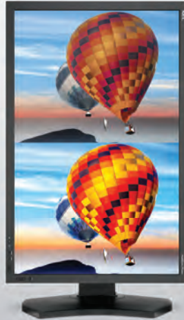
Picture by Picture shown with the same input, multiple color spaces
