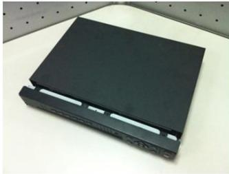
7. Put the cover in accordance with the clip and then place the upper cover back.
