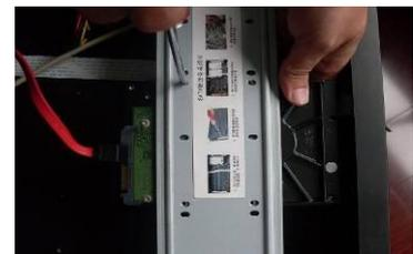
3. Use four screws to fix HDD.
