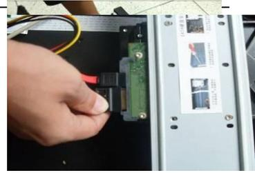
6. Connect the HDD cable and power cable.
