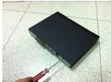
8. Secure the screws in the rear panel and the side panel.
