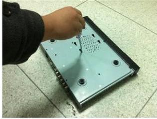
5. Fix the HDD firmly.
