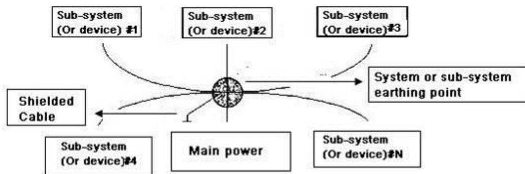
**Multiple-point ground:** In the following figure, you can see the internal circuit uses the chassis as the common point. While at the same time, all devices chassis use the earthing as the common port. In this connection, the ground structure can provide the lower ground resistance because when there are multiple-point grounds; each ground cable is as short as possible. And the parallel cable connection can reduce the total
