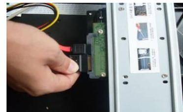
6. Insert the HDD power cable. Close the chassis and fix the screws to secure firmly.
