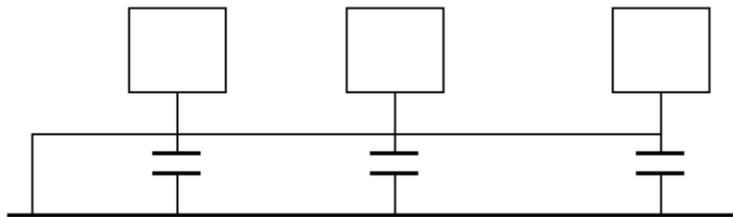
When connecting devices of huge size (the device physical dimension and connection cable is big comparing with the wave path of existed interference), then there are possibility of interference when the current goes through the chassis and cable. In this situation, the interference circuit path usually lies in the system ground circuit.
