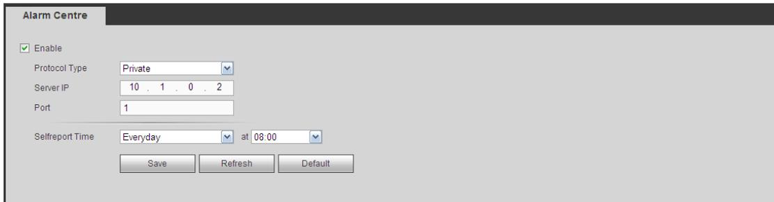
The screenshot shows the 'Alarm Centre' configuration page. It features a 'Enable' checkbox which is checked. Below it, there are several configuration fields: 'Protocol Type' is set to 'Private', 'Server IP' is '10.1.0.2', 'Port' is '1', and 'Selfreport Time' is set to 'Everyday at 08:00'. At the bottom, there are three buttons: 'Save', 'Refresh', and 'Default'.
