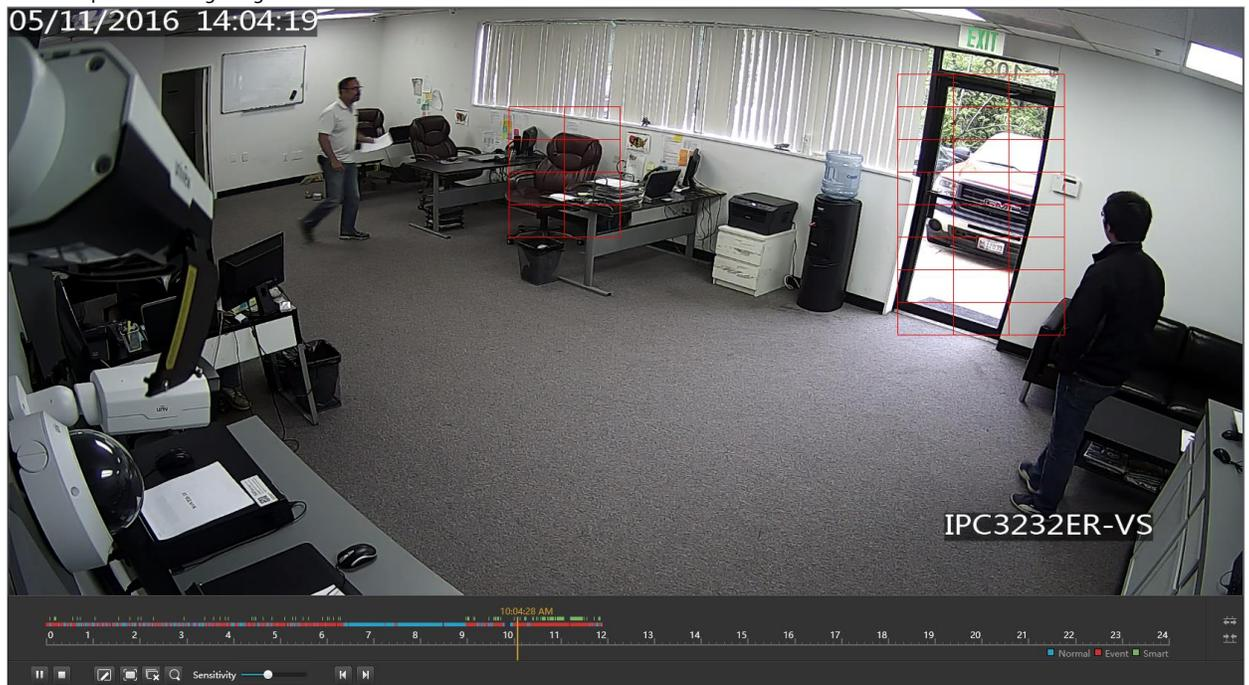
3. Once the user clicks on the search button at the bottom of the time bar the search results will narrow down and automatically start playing back only the times where there is motion in the drawn grid. It will play back the footage at a times 16 fast forward play back mode. See example of search results below.
