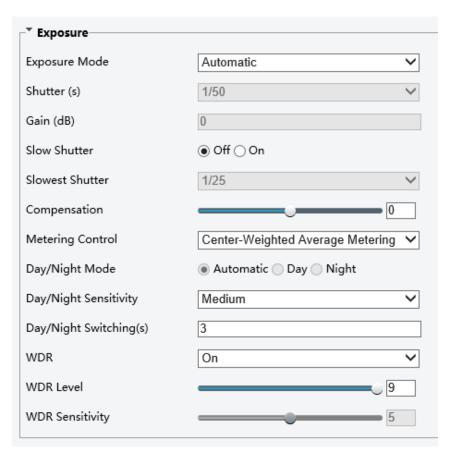
WDR Level/Sensitivity setting will be adjusted based on where the camera is installed and how much of a light difference there is. This setting will have to be changed after the camera is installed to the customer's image quality satisfaction. The higher the more range in light difference.
