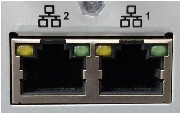
It is important that port "1" is plugged into the location's main network and port "2" is plugged into the camera network.
