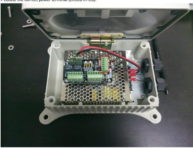
> Remove a good length of the Cat5 jacket and strip the blue and green wires. In this example, the blue wires are for video and the green is for PTZ data. Striped will be for positive (+) and solid will be for negative (-).
