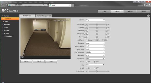
Once you have made sure that the flip is on rotate the camera lens to straighten the video out.
