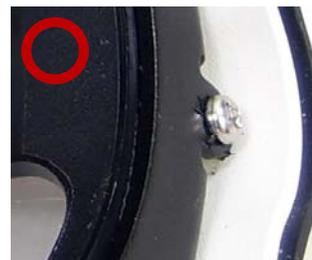
**Tightly secure the 4 screws inside the housing cover**
