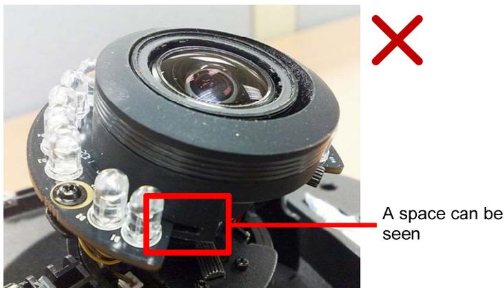
Side View: The rubber band is out of position.
