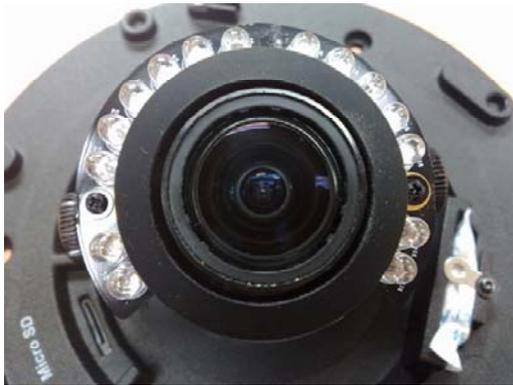
**Top view: The rubber band is at its normal position.**
