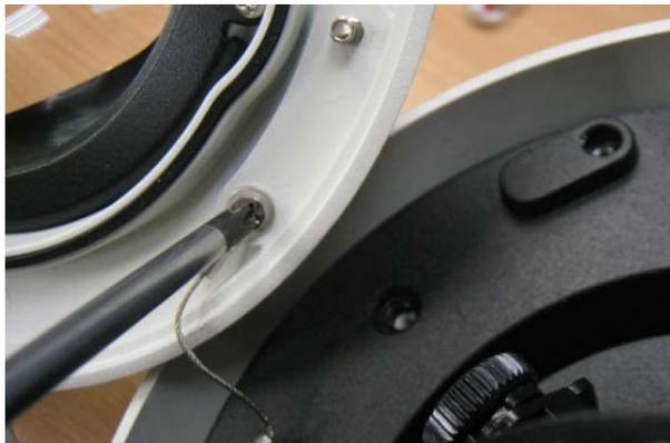
5. Unscrew the indicated parts and remove the iron ring.
