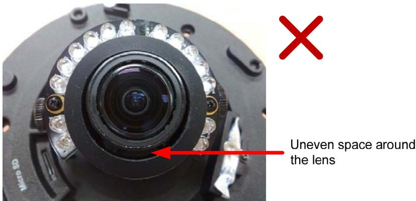
Top View: The rubber band is out of position
