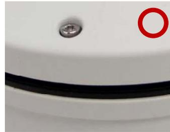
**Tightly secure the 4 screws on the housing cover**
