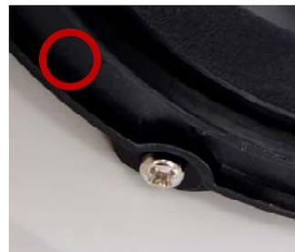
**Tightly secure the 4 screws inside the housing cover**
