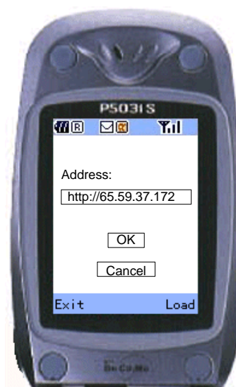
Figure 8-60 Entering the IP address of GV-server
