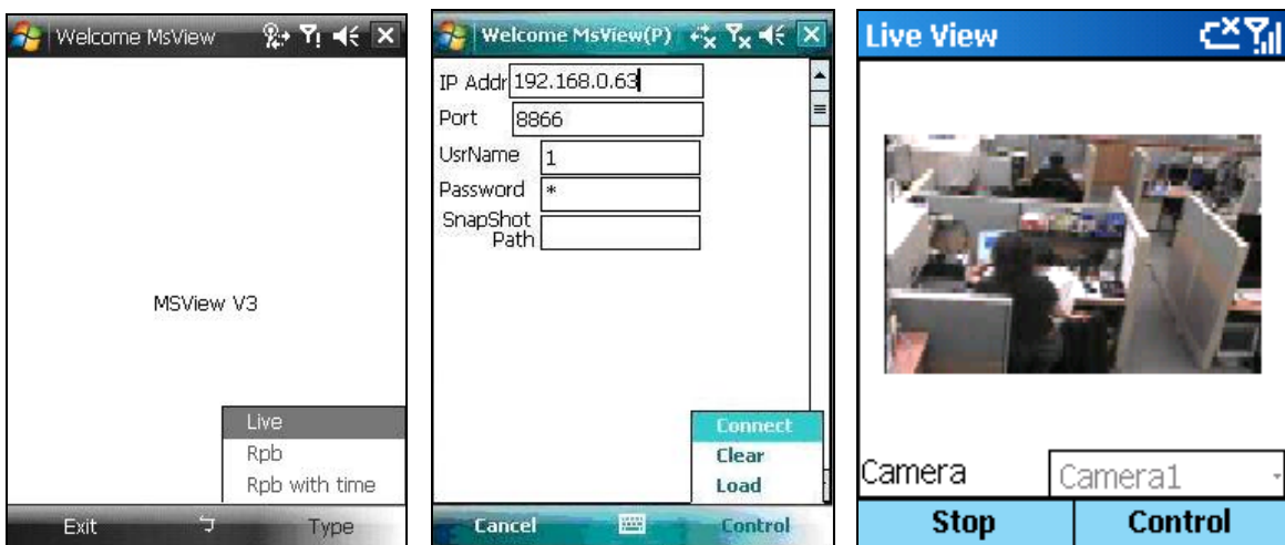
Figure 8-63 MSView Main Screen Figure 8-64 Entering GV-System Info Figure 8-65 Viewing live camera
