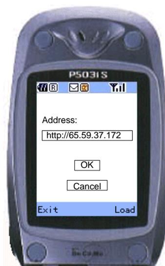
Figure 6-66 Entering the IP address of GV-server
