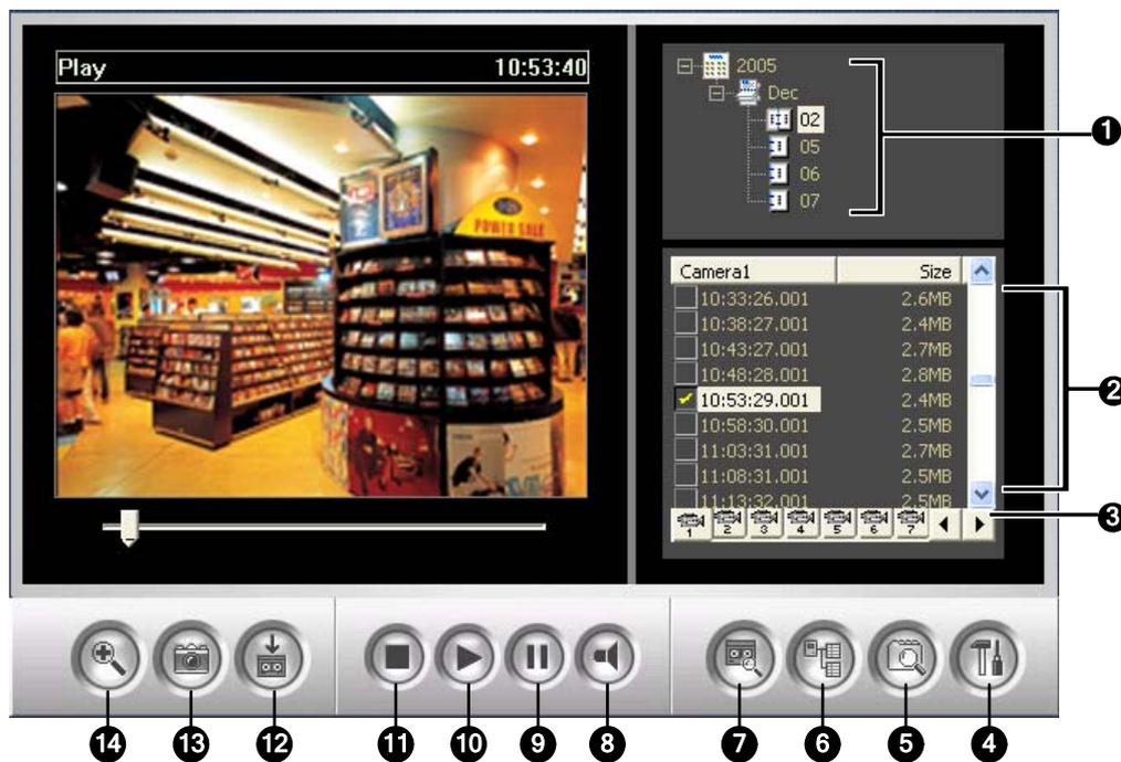
**Figure 6-44** The Remote Playback Window
