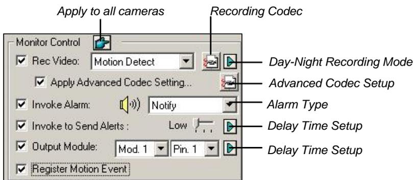
**Figure 1-13 Monitor Control Setup**
