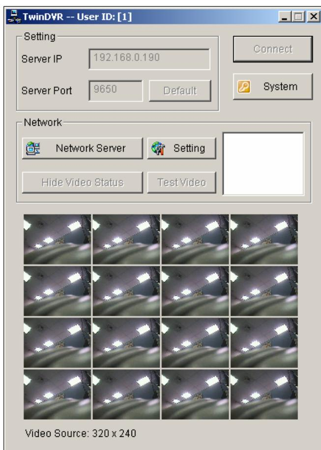
*Figure 10-9 Testing Video Stream*
