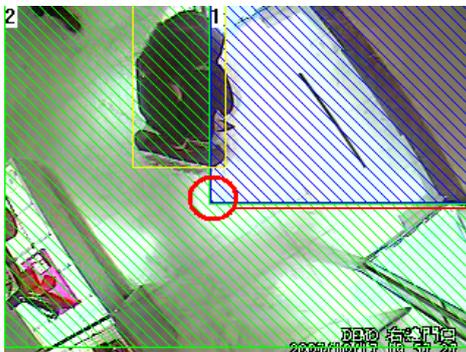
Positioning the camera in the middle of two defined detection zones.
