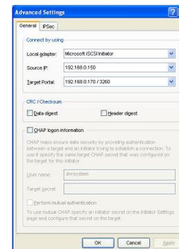
(Figure: In this example, the DVR IP address is 192.168.0.150. The iSCSI data port 1 is 192.168.0.170)
