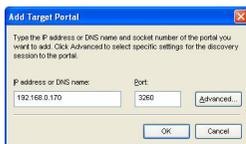
(Figure: In this example, we added iSCSI data port 1 of 192.168.0.170 and iSCSI data port 2 of 192.168.0.171 as target portals.)
