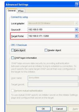
(Figure: In this example, the iSCSI data port 2 is 192.168.0.171.)
