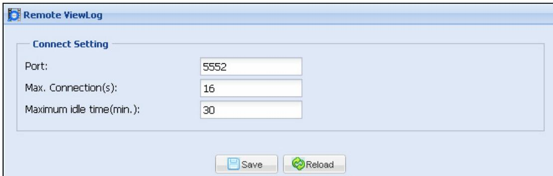
The screenshot shows a web-based configuration window titled "Remote ViewLog". Inside the window, there is a section labeled "Connect Setting" which contains three input fields. The first field is labeled "Port:" and contains the value "5552". The second field is labeled "Max. Connection(s):" and contains the value "16". The third field is labeled "Maximum idle time(min.):" and contains the value "30". Below these fields, there are two buttons: "Save" and "Reload".
