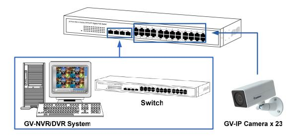
**Note:** The maximum cable length for Gigabit RJ-45 is 100 meters. For connection that exceeds 100 meters, you can use the Gigabit SFP ports.
