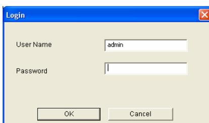
3. Type the ID and password of your GV-IP Decoder Box / GV-Pad and click **OK**. The default ID and password are **admin**. The Video Connection Setting window appears.
