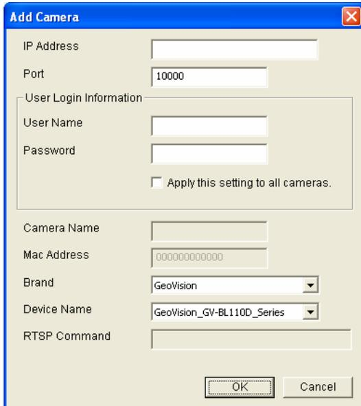
2. Type the IP address, user name and password of the device.
