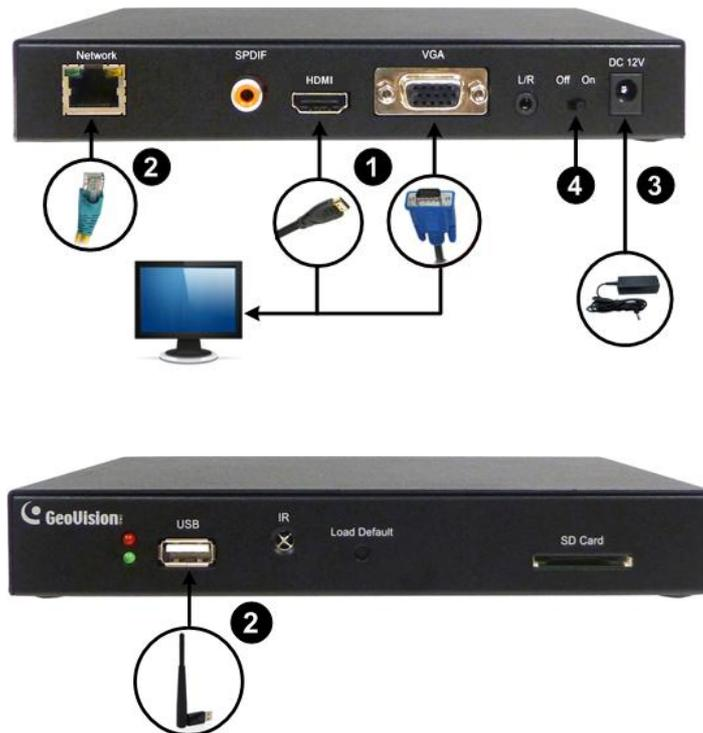
1. Connect a display device to VGA or HDMI connector for video output.
