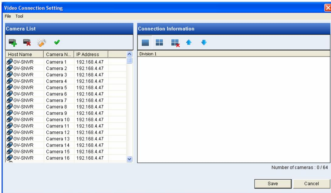
4. Use the Camera List toolbar to add, remove or configure a selected camera in the Camera List. Click the **Select All** button to select all the cameras on the list.
