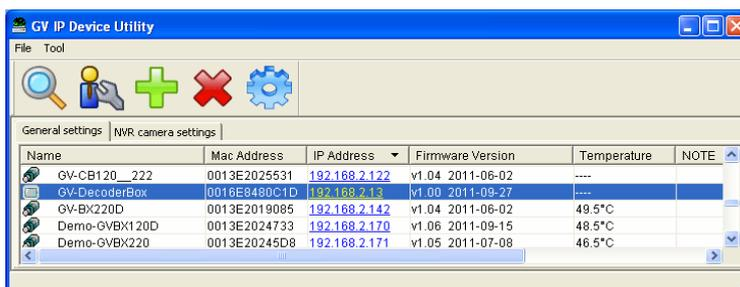
2. Double-click the IP address of your GV-IP Decoder Box / GV-Pad and select **Connect Setting**. This dialog box appears.
