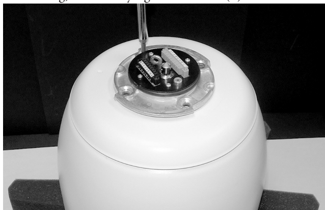
Photo 1D Replace top plate
