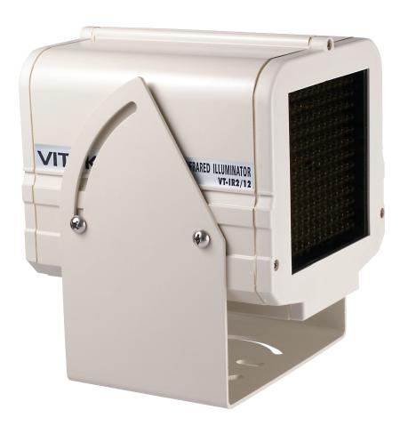
The VT-IR2/12 Infrared Illuminator is designed to enable your B/W CCD camera to deliver useable images in absolute darkness. It has range to 100 feet and runs off of low voltage 12 VDC. Heavy-duty aluminum construction and a built-in fan enable usage indoor and outdoors.
