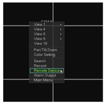
Now we must access the Remote Device menu directly on the NVR to add the remaining IP cameras. To access this menu, make sure there is a monitor and mouse connected to the NVR and using the mouse, right click anywhere on the DVR screen to bring up the menu pictured on the left. From this menu, select Remote Device. You might be asked to enter in a password. The default local username and password for our NVR systems is "888888" (without the quotes).
