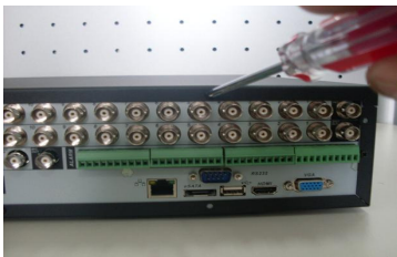
Remove the top cover from the DVR.
