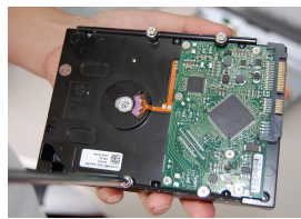
3. Loosely connect four screws to the bottom of the HDD.
