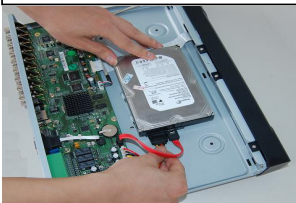
7. Connect the SATA cable and power cable.
