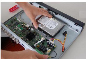
4. Mount the HDD using the four holes in the chassis.
