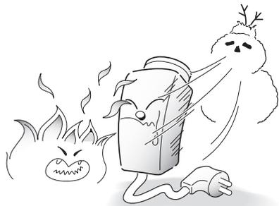
Only use the camera under conditions where temperatures are between  $-10^{\circ}\text{C}$  and  $+50^{\circ}\text{C}$ . Be especially careful to provide ventilation when operating under high temperatures.
