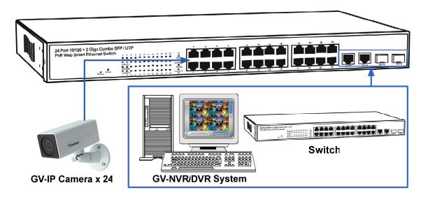
**Note:** The maximum cable length for Ethernet is 100 meters. For connection that exceeds 100 meters, you can use the Gigabit SFP ports.
