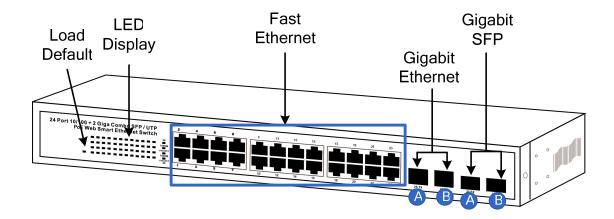
**Important:** For the usage of Gigabit Ethernet and Gigabit SFP ports, you can only choose one port from group A and one port from group B to connect. Both groups offer one of their ports for connections at a time.
