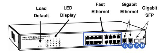
**Important:** For the usage of Gigabit Ethernet and Gigabit SFP ports, you can only choose one port from group A and one port from group B to connect. Both groups offer one of their ports for connections at a time.
