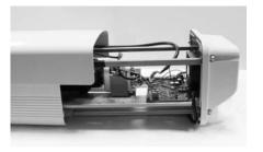
. Secure the camera enclosure with the screws on both sides.
